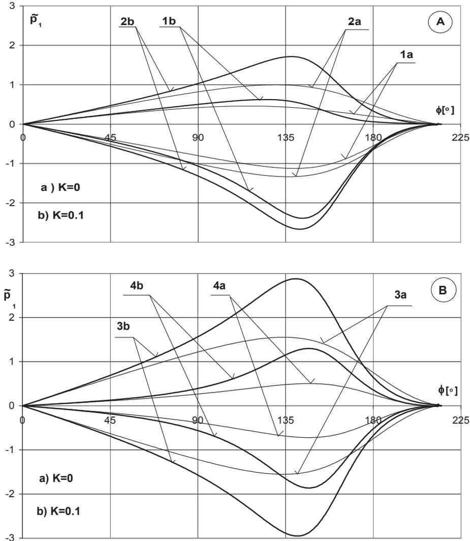
Fig. 2. Unsteady part maximal and minimal pressure distributions  $\tilde{p}_1$  in direction  $\phi$  a) for constant oil viscosity ( $K=0$ ), b) for oil viscosity in dependence on pressure ( $K=0.1$ ) by velocity perturbations: 1)  $V_{10}=0.05$ ;  $V_{1h}=0$ ; 2)  $V_{10}=0.05$ ;  $V_{1h}=0.025$ . 3)  $V_{10}=0.05$ ;  $V_{1h}=0.05$ ; 4)  $V_{10}=0.05$ ;  $V_{1h}= - 0.05$
