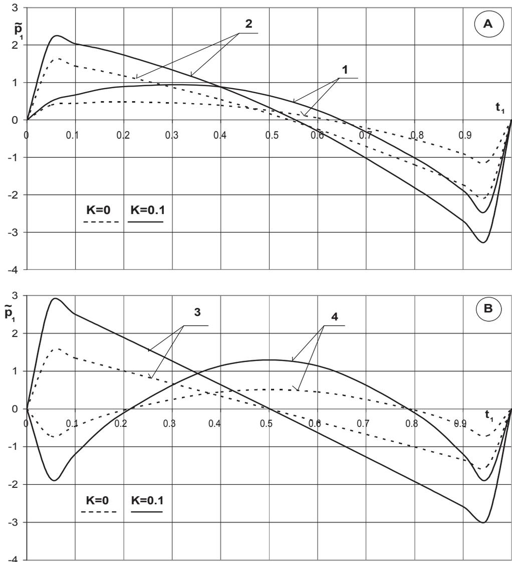
Fig. 1. Pressure distributions  $\tilde{p}_1$  in place  $\varphi=145^\circ$  in the time  $t_1$  for constant oil viscosity ( $K=0$ ) and for oil viscosity in dependence on pressure ( $K=0.1$ ) by velocity perturbations: 1)  $V_{10}=0.05$ ;  $V_{1h}=0$ ; 2)  $V_{10}=0.05$ ;  $V_{1h}=0.025$ ; 3)  $V_{10}=0.05$ ;  $V_{1h}=0.05$ ; 4)  $V_{10}=0.05$ ;  $V_{1h}=-0.05$
