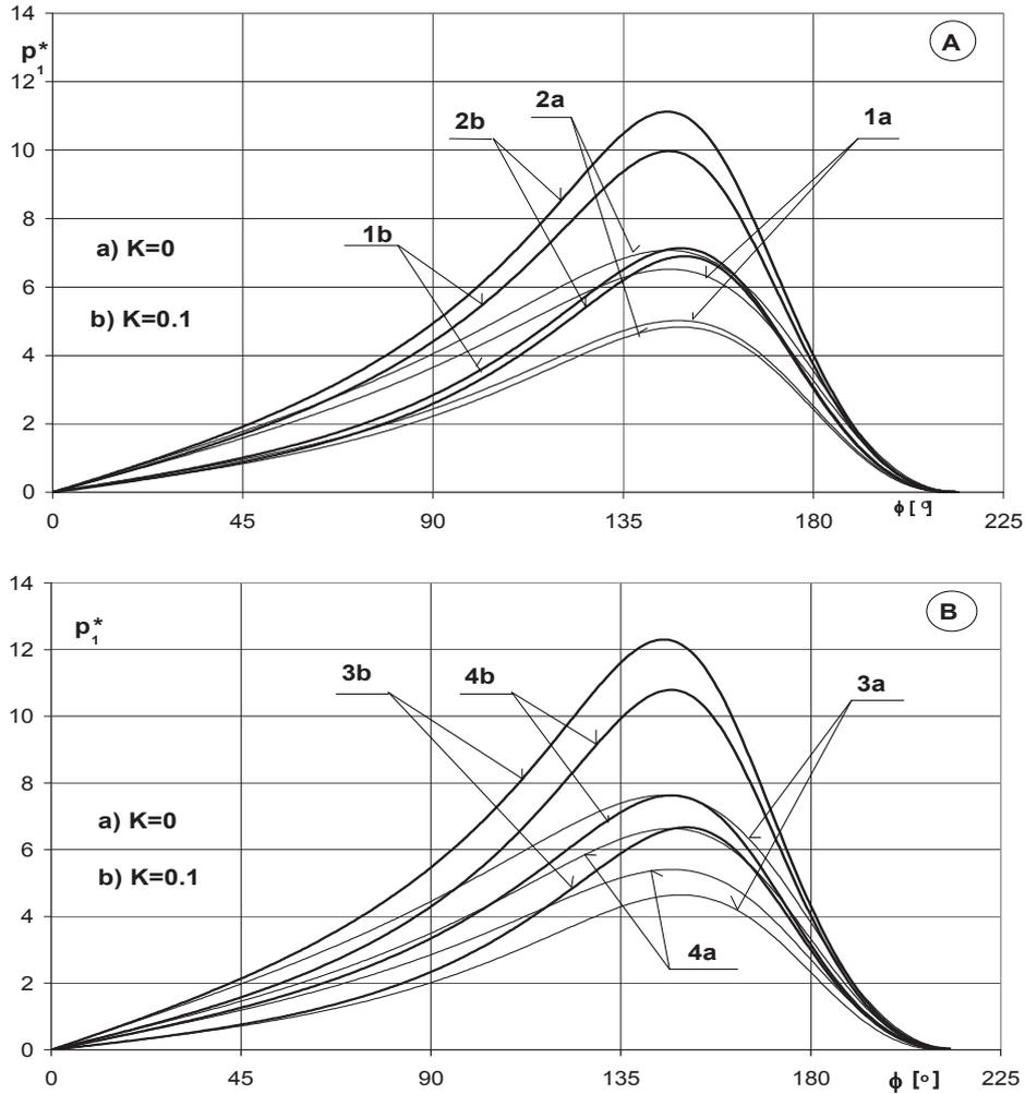
Fig. 3. Total maximal and minimal pressure distributions  $p_1^*$  in direction  $\phi$  a) for constant oil viscosity ( $K=0$ ) and b) for oil viscosity in dependence on pressure ( $K=0.1$ ) by velocity perturbations: 1)  $V_{10}=0.05$ ;  $V_{1h}=0$  2)  $V_{10}=0.05$ ;  $V_{1h}=0.025$ . 3)  $V_{10}=0.05$ ;  $V_{1h}=0.05$ ; 4)  $V_{10}=0.05$ ;  $V_{1h}=-0.05$
